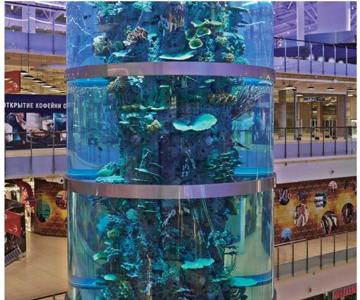
*The aquarium at the Avia Park shopping center in Moscow, Russia is a record-breaking 75 feet tall. The tank is constructed of seven sections of R-Cast® acrylic, which weigh up to 26,000 pounds each. The acrylic is eight inches thick in order to retain the 98,000 gallons of water within the tank. Photo courtesy of Reynolds Polymer Technology, Inc.*
